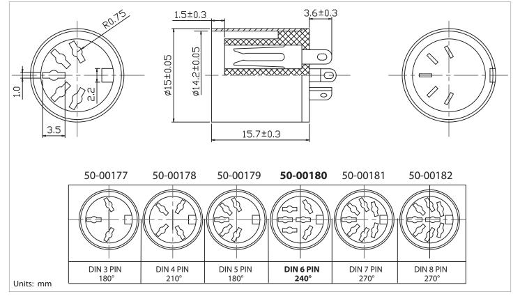
tolerance X: ±0.5 mm .X: ±0.3 mm .XX: ±0.05 mm applicable unless otherwise indicated in specification or on drawings
