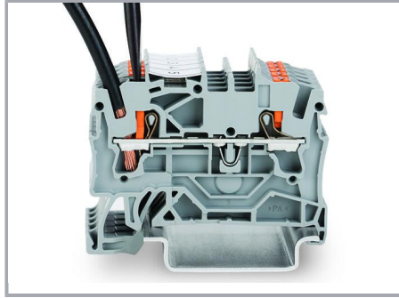
Removing all conductors via operating tool.
