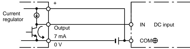
NPN open-collector output
