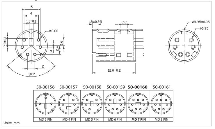
tolerance X: ±0.5 mm .X: ±0.3 mm .XX: ±0.05 mm applicable unless otherwise indicated in specification or on drawings
