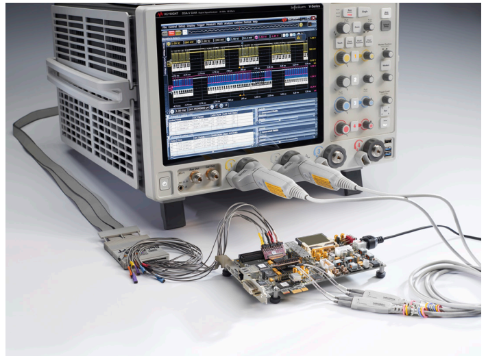
DDR3 test setup with mixed signal oscilloscope.
