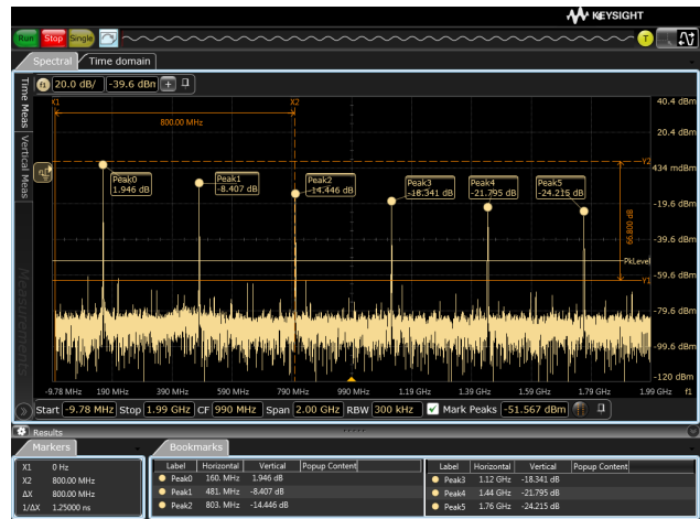
Peak readouts in the FFT plot.
