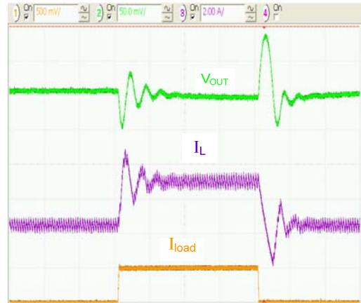
Figure 14. 500 mA to 3 A to 500 mA, 5 \mu\text{s}/\text{div} .
