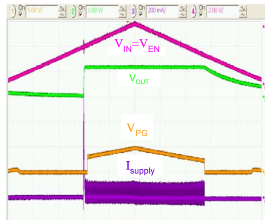
Figure 18. Soft-Start, EN Pin Tied to VCC I_{LOAD}=0 , 1 ms/div.
