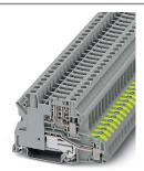
Ground modular terminal block, nom. voltage: 500 V, nominal current: 20 A, connection method: Screw connection, Rated cross section: 2.5 mm², cross section: 0.14 mm² - 6 mm², mounting: NS 35/7,5, NS 35/15, color: gray
