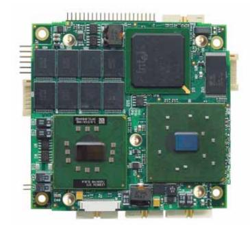
The CPU-1484 is an embedded RoHS compliant board based on two modules: a mezzanine CPU module combined with a PC/104-Plus form factor carrier.
