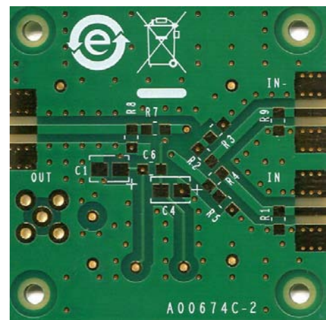
Figure 2. Circuit Side of Evaluation Board
