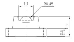
For reflow soldering (propose)
