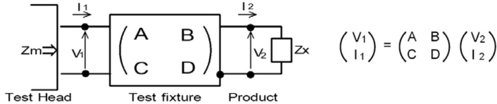
(2) The product's impedance value (Zx) and measured impedance value (Zm) can be expressed as shown below, by using the respective current and voltage for input/output.
