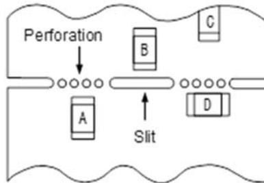
(3) Mounting components near screw holes
