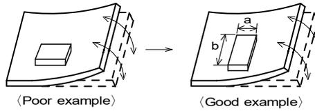
(2) Components location on PCB separation
