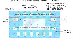
NOTE: 1. COPLANAR WAVEGUIDE PARAMETERS ARE SHOWN FOR ROGERS RO4350B WITH DIELECTRIC THICKNESS .060"±.004"; COPPER: 1/2 Oz. EACH SIDE. FOR OTHER MATERIALS TRACE WIDTH MAY NEED TO BE MODIFIED.
