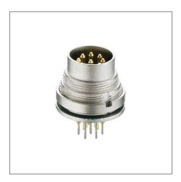
Chassis plug acc. to AISG specification and IEC 61076-2-106, IP 68, with threaded joint, for printed circuit boards, for back side mounting
