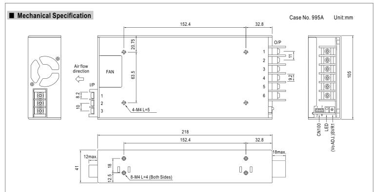
AC Input Terminal Pin No. Assignment
