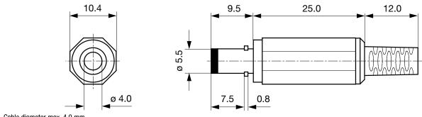
Cable diameter max. 4.0 mm
