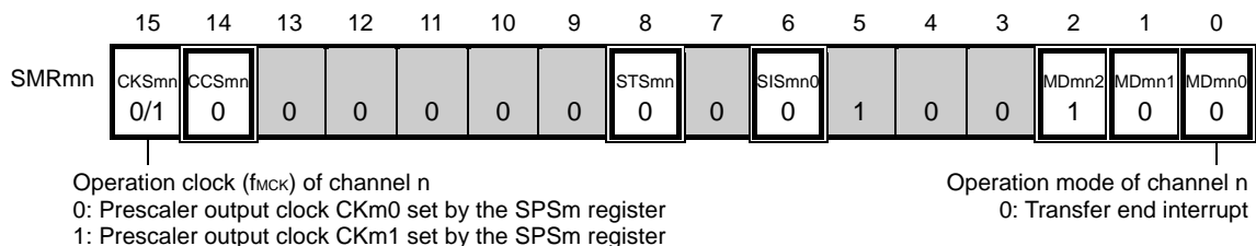
Figure 13-117. Example of Contents of Registers for Address Field Transmission of Simplified I 2 C (IIC00, IIC01, IIC10, IIC11, IIC20, IIC21)(1/2)
