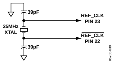
Figure 40. Crystal Configuration for Reference Clock Source
