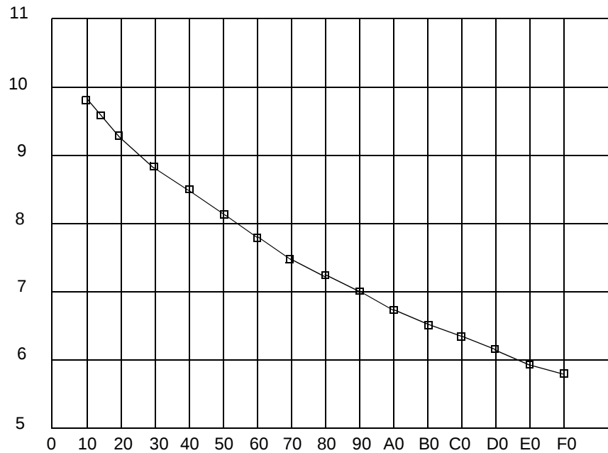
Figure 10. Typical Relaxation Oscillator Frequency vs. Trim Value @ 25°C
