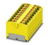
Distribution block, bridged internally, nom. voltage: 450 V, nominal current: 32 A, connection method: Pushin connection, number of connections: 18, cross section: 0.2 mm<sup>2</sup> - 6 mm<sup>2</sup>, AWG: 24 - 10, width: 55.4 mm, height: 21.7 mm, color: yellow, mounting type: for snapping onto a DIN rail adapter, for snapping onto a DIN rail adapter, Adapter plate
