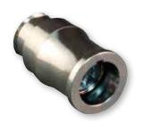
Series 880 Quick-Disconnect (QDC) in-line receptacles with solder cup contacts have thread-on rear adapter to allow access to contacts. Install cable shield braid directly to connector with Band-Master® band. Three contact sizes are available with current ratings of 5A, 3A and 1A. Aluminum or stainless steel housings and thermoplastic insulators. Ultraminiature SuperFly® connectors are ideal where ruggedness and field repairability is required.
