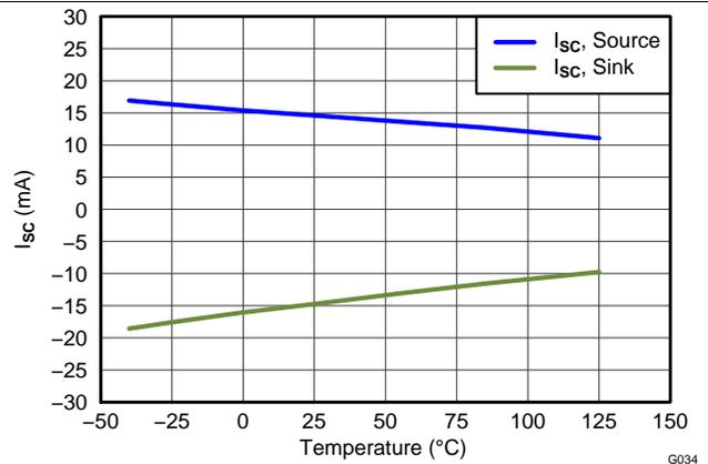
Figure 34. Short-Circuit Current vs Temperature
