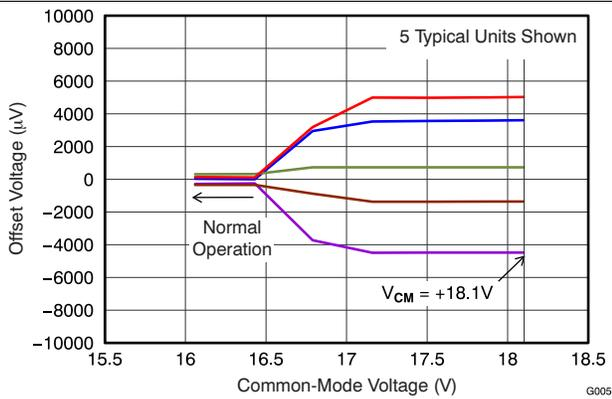
Figure 5. Offset Voltage vs Common-Mode Voltage (Upper Stage)
