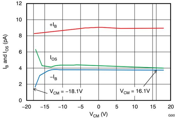
Figure 7.  $I_B$  and  $I_{OS}$  vs Common-Mode Voltage
