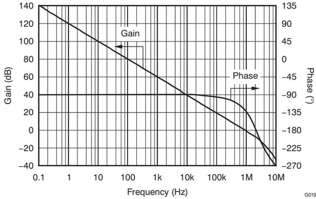
Figure 19. Open-Loop Gain and Phase vs Frequency
