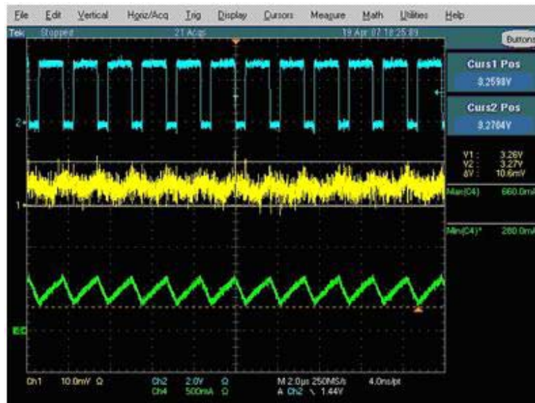
Figure 9. Ceramic 22 \mu F 1210(X5R) (Good)
