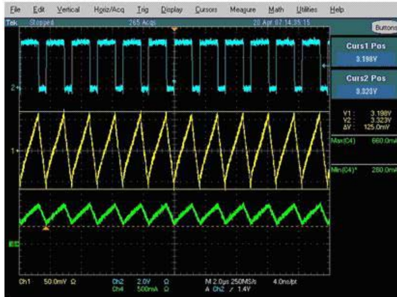
Figure 11. Electrolytic 100 \mu F (Ripple Too High)
