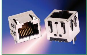
Bel Stewart's SS-60300 Series CAT6a jacks are designed for use in CAT6a patch panels and wall outlets in premise wiring systems. Engineered to meet the 500 MHz requirements of the CAT6a specifications, the SS-60300 jacks provide a higher level of compensation to reach defined performance levels.
