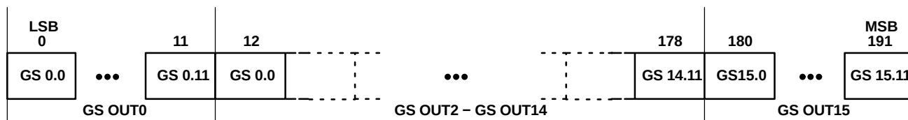
Figure 9. Grayscale Data Packet Format
