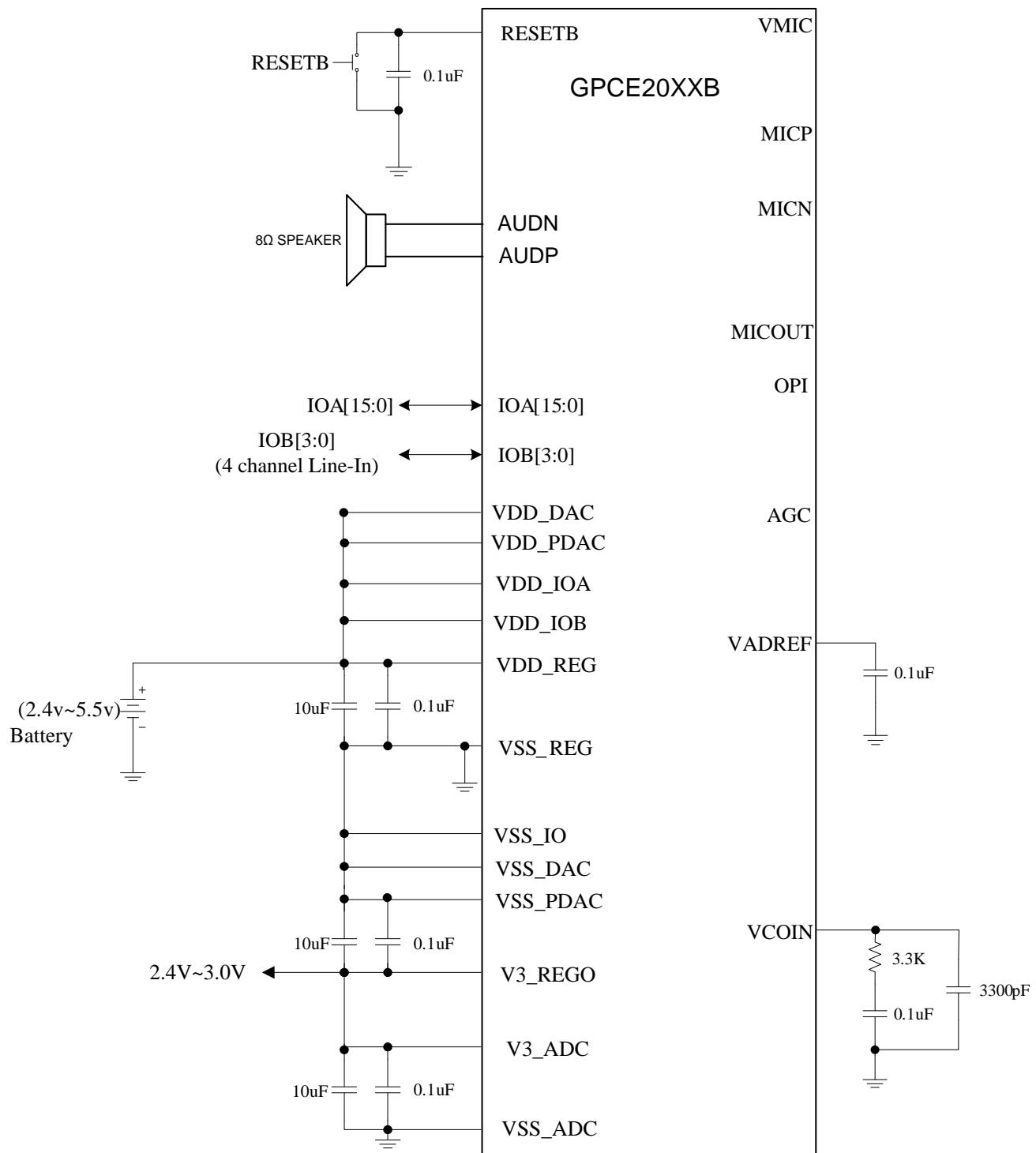
**Note:** V3\_REGO is output of built-in regulator with maximum current 40mA. It is recommended that only use it for internal power pad.
