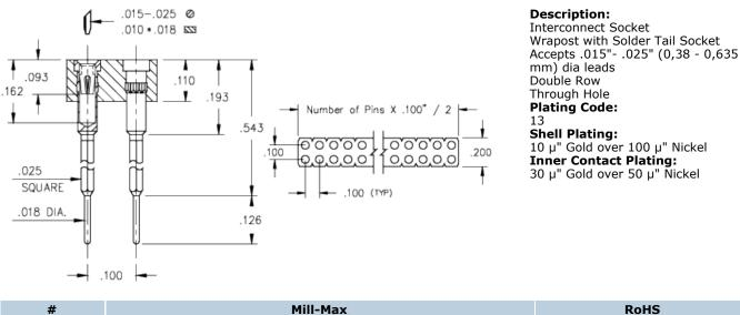
Shell Plating: 10  $\mu$ " Gold over 100  $\mu$ " Nickel Inner Contact Plating: 30 µ" Gold over 50 µ" Nickel
