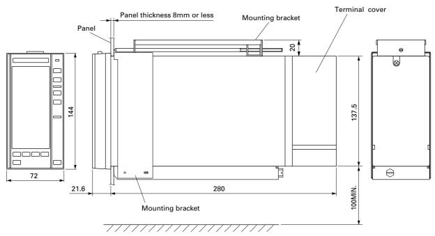
Note) The distance between other instruments and low end of PDG shall be more than 100mm.
