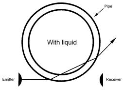
If the diameter of the pipe is close to 6 mm, some of the emitted light may reach the receiver because the angle of refraction is small. This may result in false readings. In such cases, set the sensitivity selector to Low and check that the EE-SPX613 reads correctly for pipes with and without liquid.
