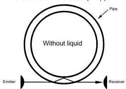
2. If there is liquid in the pipe, the emitted beam will pass through the liquid and not reach the receiver.
