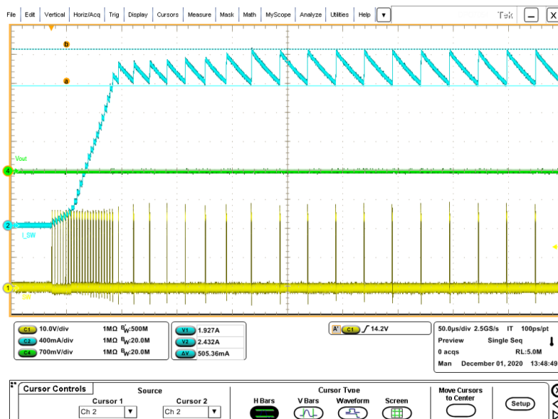
Figure 21. Soft-start procedure with VOUT shorted to GND
