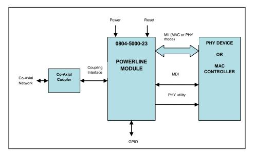
The block diagram presents the 0804-5000-23 powerline module in a typical environment. Seven different types of interfaces are shown. These interfaces are described in detail below.
