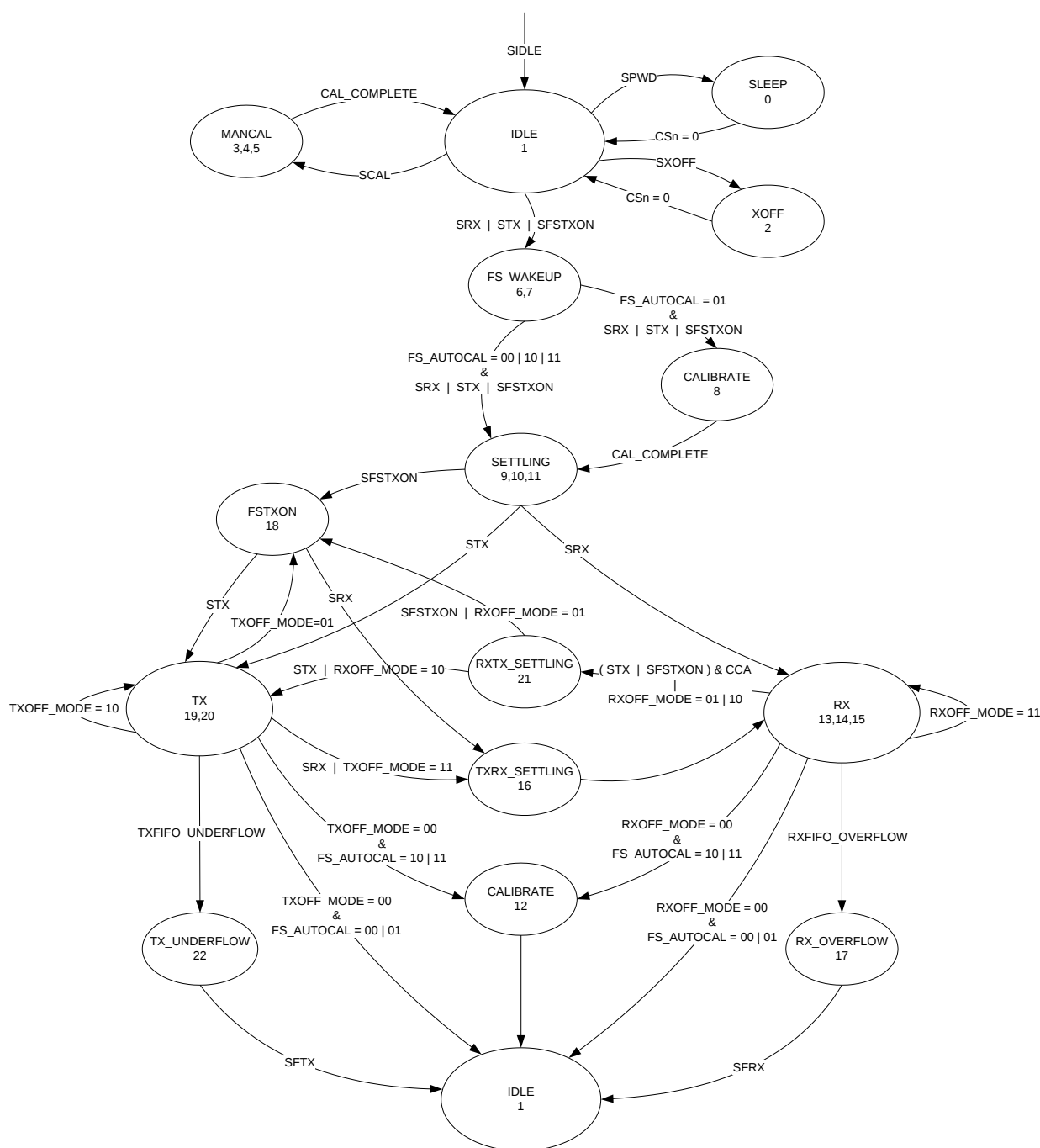
Figure 19: Complete Radio Control State Diagram
