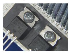
Sil-Pad® 1200 is a silicone based, fiberglass-reinforced thermal interface material featuring a smooth, highly compliant surface. The material features a non-tacky surface for efficient re-positioning and ease of use, as well as an optional adhesive coating. Sil-Pad® 1200 exhibits exceptional thermal performance at low and high application pressures. The material is ideal for placement between electronic power devices and a heatsink for screw and clip mounted applications.
