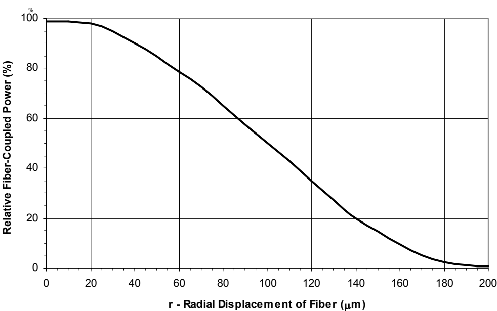
Figure 4 - Relative Fiber-coupled Power vs. r - Radial Displacement of Fiber
