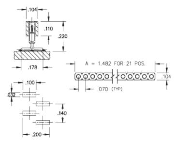
Interconnect Socket Surface Mount Socket Accepts .015"- .025" (0,38 - 0,635 mm) dia leads Single Row Surface Mount Plating Code: Shell Plating: 200 μ" Tin/Lead(93/7) over 100 μ" Nickel Inner Contact Plating:
