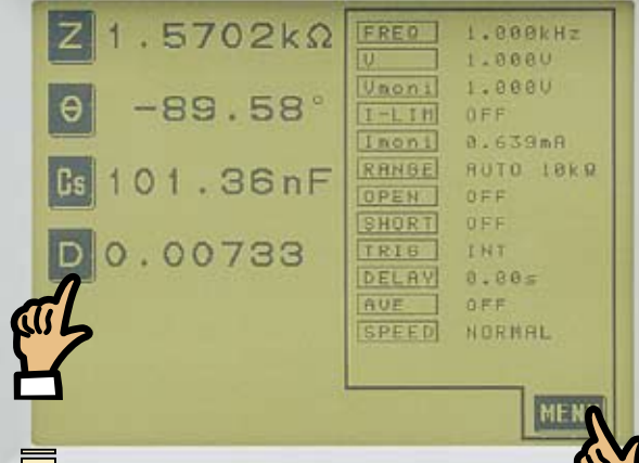
Initial screen Shows measurement values for any selected four parameters, and current settings of conditions.
