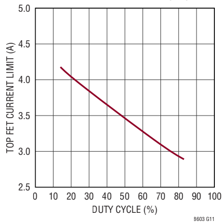
Channel 2 Peak Current Limit vs Duty Cycle
