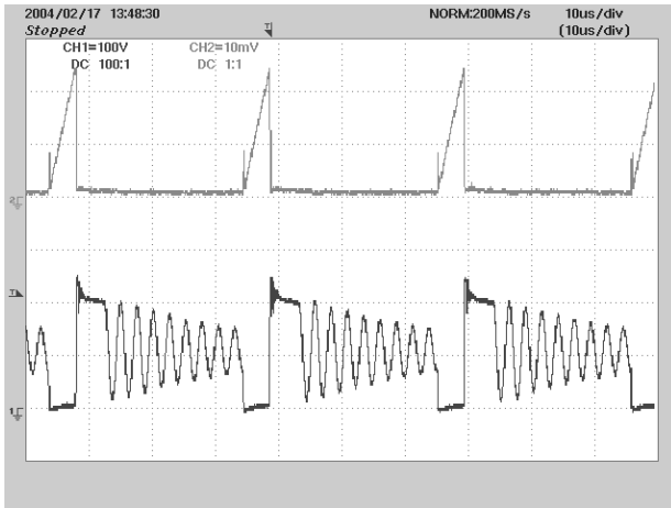
Figure 8 - 85 VAC, Full Load. Upper: I_{DRAIN} , 0.1 A / div Lower: V_{DRAIN} , 100 V, 10 \mu s / div
