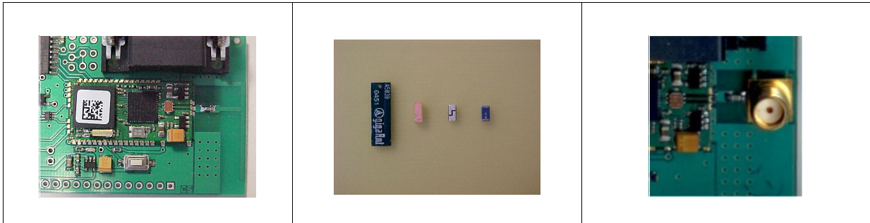
Figure 5. SMA connector for external antenna
