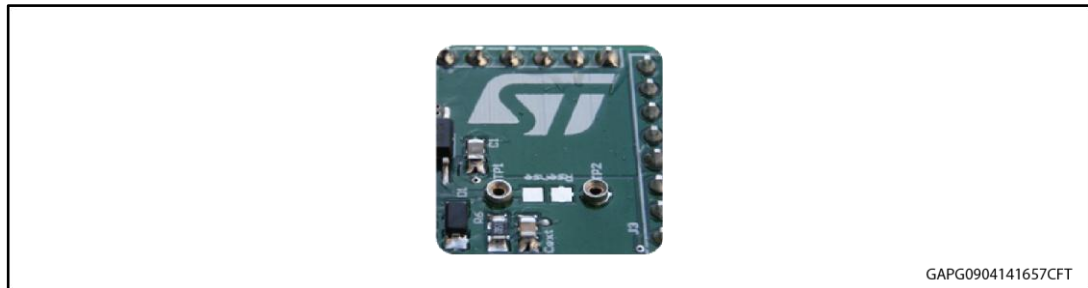
Figure 4: Mounting through-hole sense resistor
