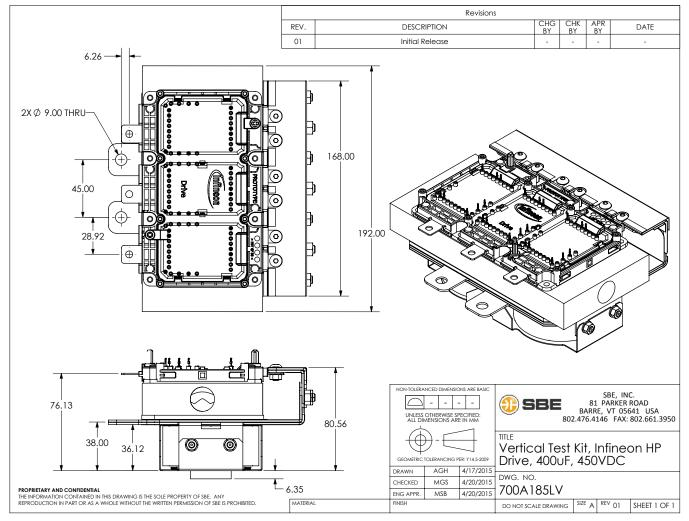
Note: HP Drive Module and Cooling Plate Not Included
