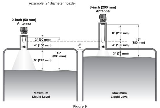
Using nozzle height to maximize useable tank space
