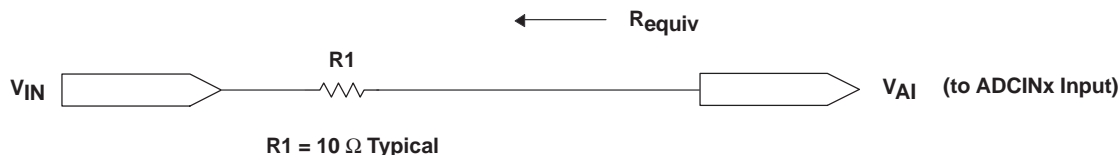
Figure 41. Typical ADC Input Pin Circuit
