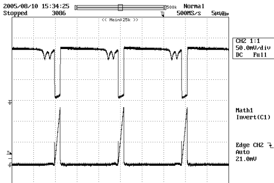
Figure 5 - 85 VAC, Full Load. Upper: I_{DRAIN} , 50 mA / div Lower: V_{DRAIN} , 50 V, 5 \mu s / div
