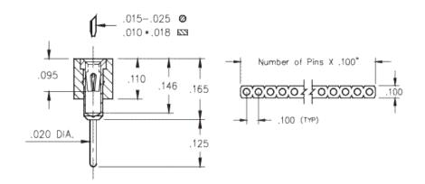
**Description:** Interconnect Socket Standard Solder Tail Socket Accepts .015" - .025" (0,38 - 0,635 mm) dia leads Single Row Through Hole Plating Code:
