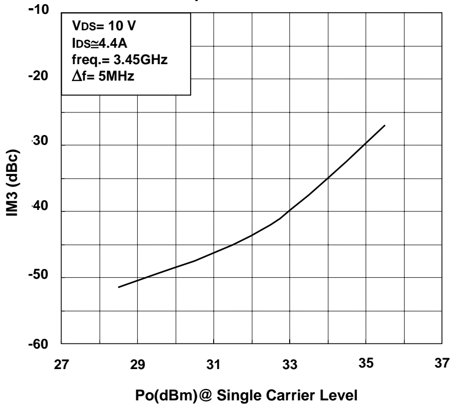
IM3 vs. Output Power Characteristics
