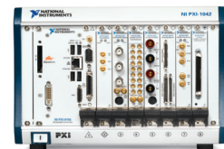
Figure 1. This NI PXIe-8106 controls an 8-slot PXI Express modular instrument and data acquisition system.
