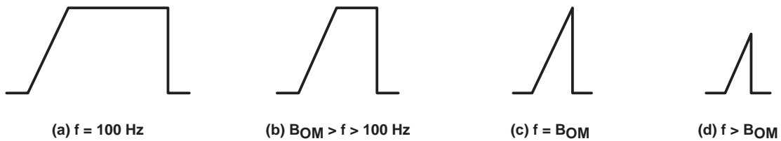
Figure 5. Full-Power-Response Output Signal
