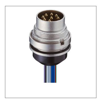
Chassis plug acc. to IEC 61076-2-106 and AISG specification, IP 68, with threaded joint, cables and potted solder area, for back side mounting
