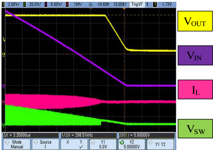
Figure 23. Shut-Down Transition at No Load
