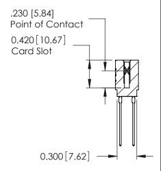
ACAD REFERENCE NO. 725-ENG MASTER 725 Series Ultra-Mate Card Edge Connector - Press Fit DRAWN: J.LEE DATE: AUG31/09 Part Number: 725-016-541-201 SEGTION A-A CHECKED: SHEET 1 OF 1 **EDAC INC** SCALE: THESE DRAWINGS AND SPECIFICATIONS ARE THE PROPERTY OF EDAC INC.,AND TORONTO, ONTARIO SHALL NOT BE REPRODUCED, OR COPIED DRAWING NUMBER **ISSUE** CANADA OR USED AS THE BASIS FOR THE 725-ENG MASTER MANUFACTURE OR SALE OF APPARATUS YOUR CONNECTION TO QUALITY & SERVICE WITHOUT WRITTEN PERMISSION.
